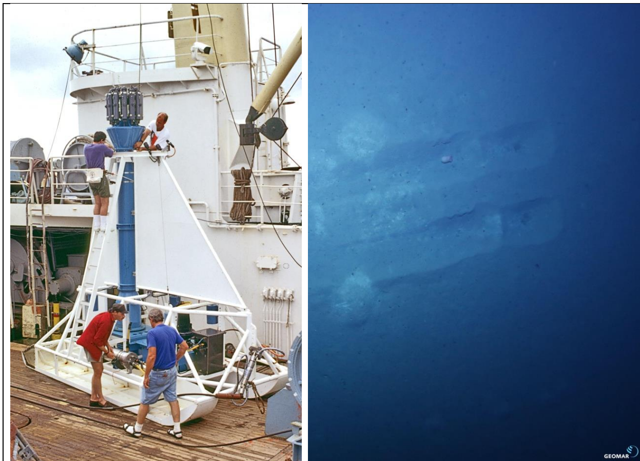
Fig. 1: Das Deep Sea Sediment Resuspension System „DSRS“ an Bord des FS Yuzhmorgeologiya in 1995 (links) , begin einer Spur, augenommen von AUV (rechts). The Deep Sea Sediment Resuspension System „DSRS“ on board RV Yuzhmorgeologiya in 1995 (left), start of trawl with this gear , photographed by the AUV (right).
