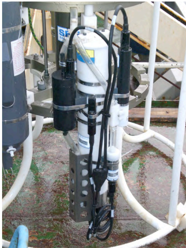
Fig. 60: Oceanographic probe SBE 19plus SEACAT Profiler equipped with sensors for measuring water turbidity, dissolved oxygen concentration and fluorescence.
