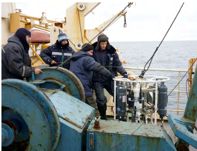
Fig. 59: CTD probe SBE 19+ attached to a programmable rosette SBE 32C with 5-liter plastic water-sampling bottles with a release for the opening of water-sampling bottles at certain depth levels (Auto Fire Module).
