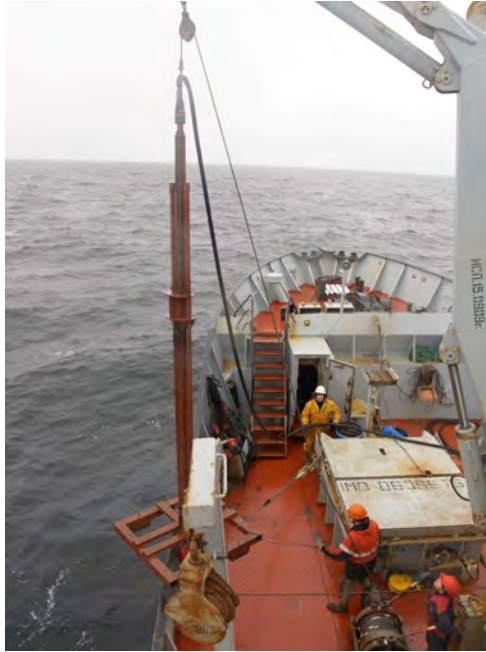
Fig. 26: The MVD is taken outboard with the help of cargo crane and winch.
