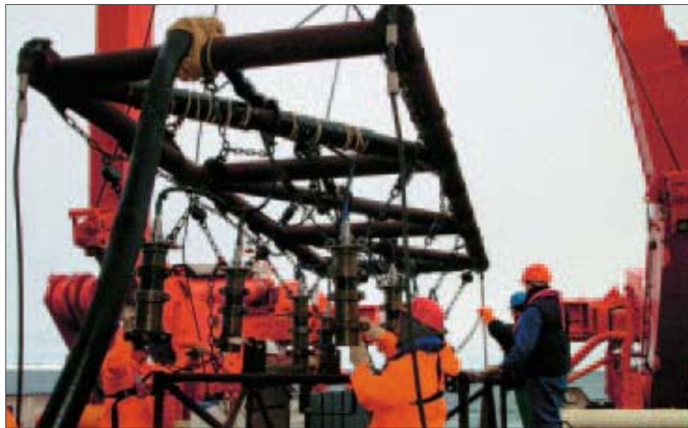
Smaller-sized air guns towed through the ice behind the ship generate acoustic signals to obtain geophysical reflections. Above: Gigantic ice flows with blue pools of melt water. The weathered surface is typical of the summer. Right: A TV-controlled "grab" brings samples up to the surface from the ocean floor.
