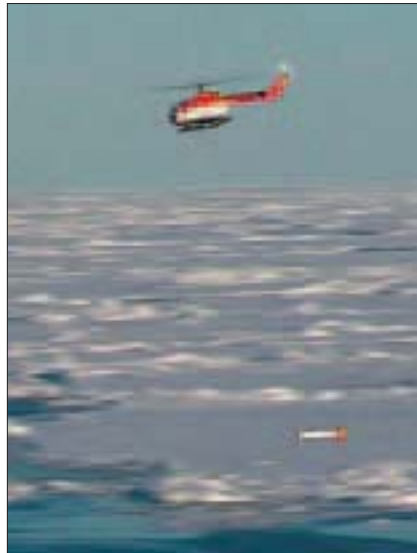
A helicopter flying at an altitude of 20 metres measures the thickness of the ice cover beneath it using a helicopter electromagnetic probe ("HEM-Bird"). Left: Magnetic fields are also probed. Above: A basalt sample from the ocean floor. The "giant pillow" weighs several tonnes.
