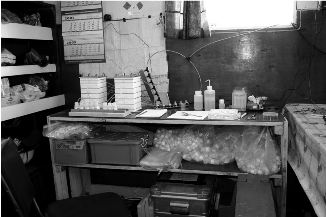
Figure 11: Pore water press in use in the field to extract sediment pore water
