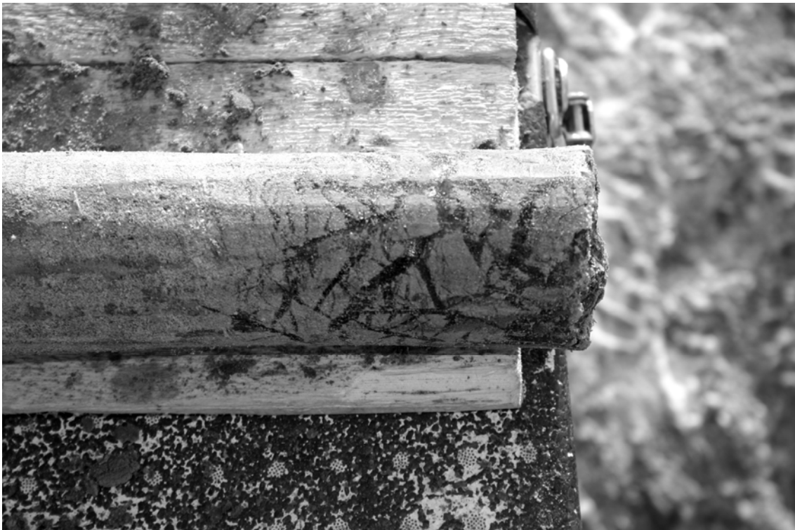
Figure 12: Detail photograph of core C-2 taken in the field. Although recovered from a submarine environment, ice-rich, terrestrial cryogenic structures are visible, indicating the occurrence marine transgression and/or coastal erosion
