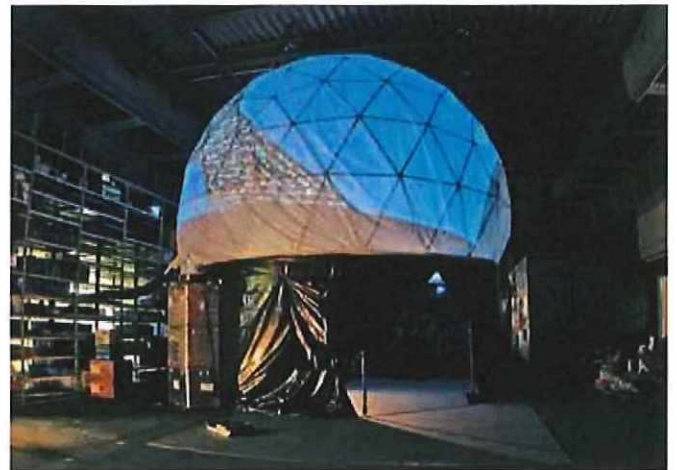
Left: Test assembly of the support structure. Note the modular foundation ring at the base. Correct dimensions were validated using a theodolite. Right: Rear projection test without the inner canvas. Note the projector (on boxes) and the evacuation nozzle at left. The dome rests on 10 vertical metal struts of 2m length. The projection (one channel active) is calibrated for 180° FoV. All photos by and/or courtesy the author.
