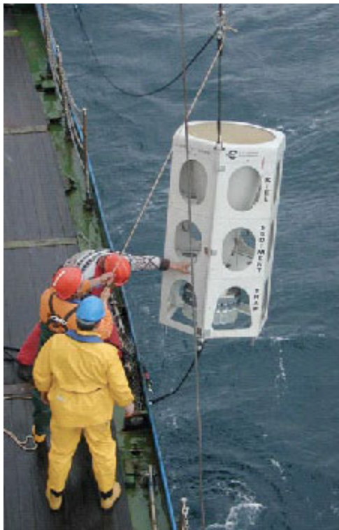
Fig. 12. Deployment of a sediment trap mooring from the Bremen Group.
