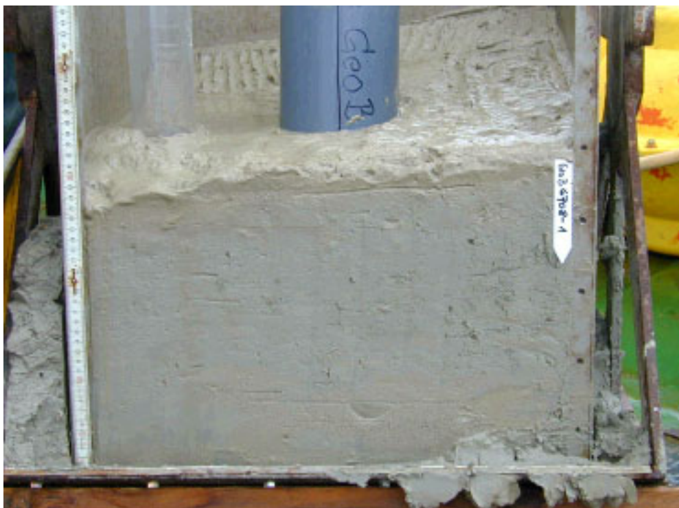
Fig. 31. Opened GKG GeoB 6708-1 with a light brownish grey slightly sandy mud on top and an olive grey silty clay, which is much stiffer than the overlying layer beneath.
