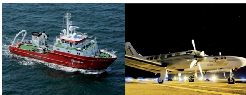
Fig. 1: A typical modern dedicated survey vessel for hydrographic data acquisition (MV »Fugro Helmert«) and a typical airborne LiDAR bathymetry aircraft
