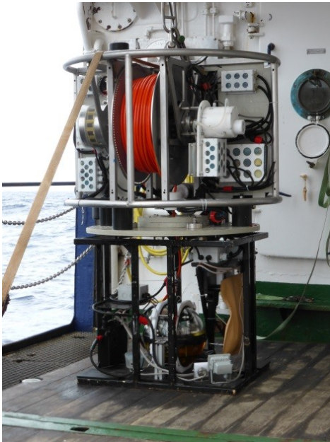
Figure 4: Buoyancy trim system under TMS ready for deployment.
