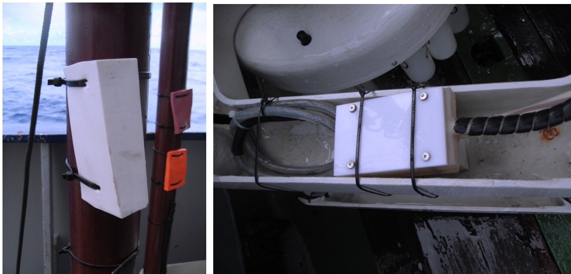
Figure 6: Pressure neutral samples on sediment trap after two years into 3000 m depth.
