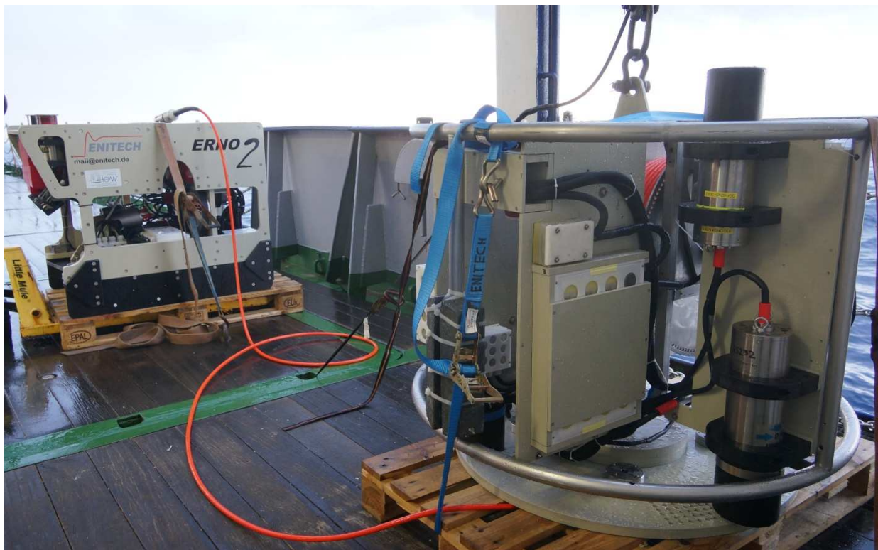
Figure 2: ERNO2 ROV and TMS docking station 2012 separated on deck
