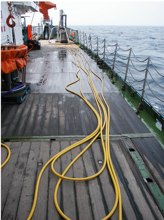
Fig. 16. Preparation for ROV deployment. The first 100 m of tether were placed on deck the RV Poseidon.
