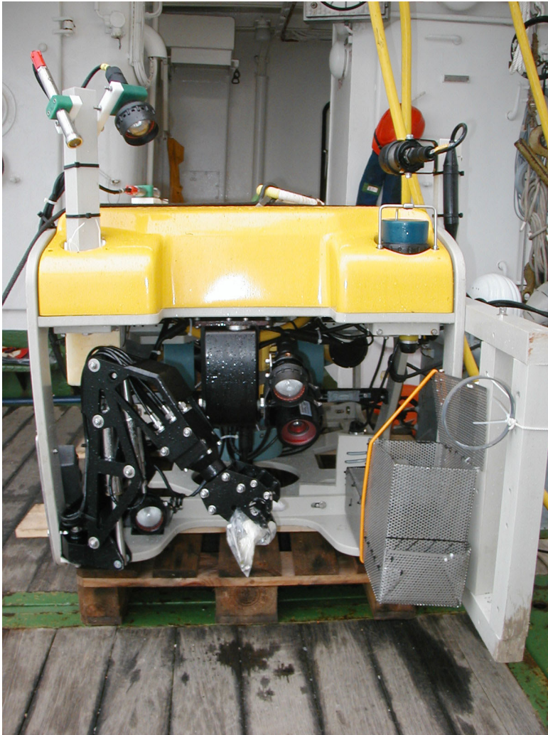
Fig. 15. Front view of the Cherokee ROV. Visible the TRITECH pilot cam (middle), HYDROLEK manipulator (left), JAI cam #1 with add. light (left), scanning sonar head (blue cap right) and the sample box (right).
