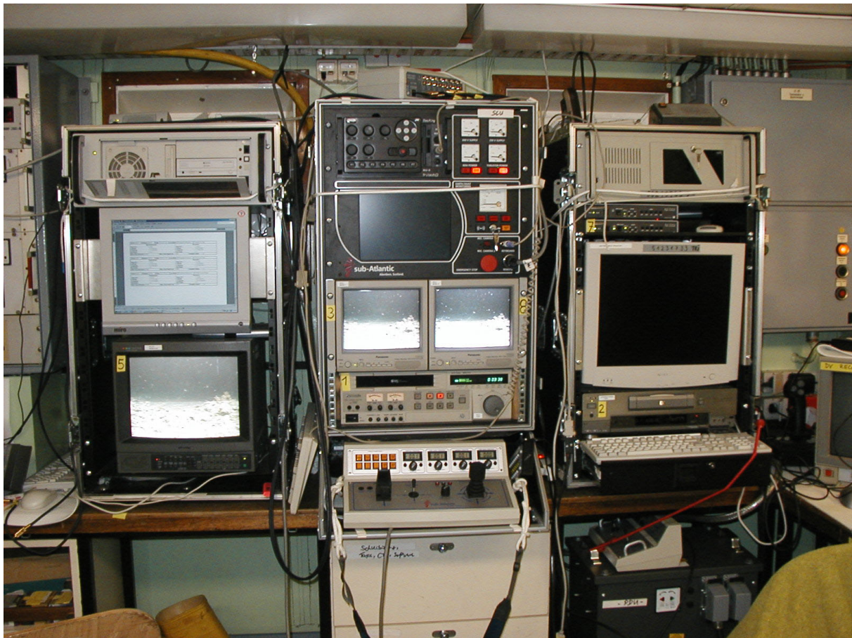
Fig. 12. Surface control unit (SCU, middle) with the additional pilot rack (PR, left) and the stereo rack (SR, right).
