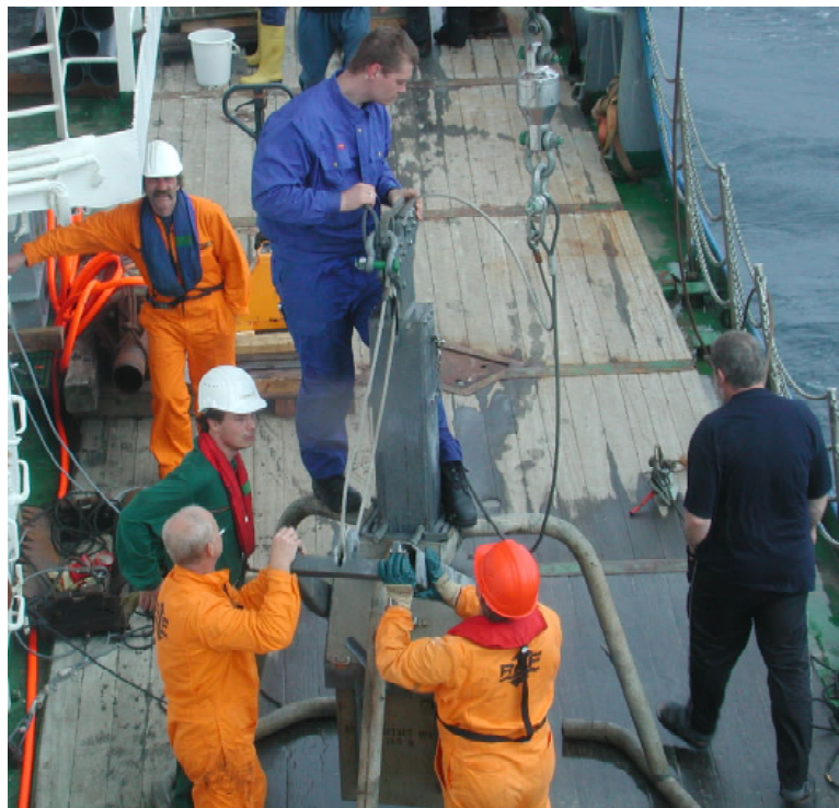
Fig. 4. On the way to Propeller Mound: Maintenance work on the heavily used box corer
