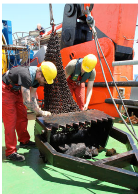
Fig. 4.9.1-2: Rock corer. The shattered pieces of rock stick to the small containers, which are filled with Vaseline and demonstrate a successful sampling of the volcanic crust.
