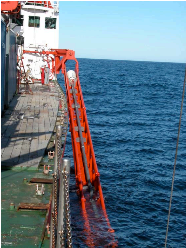
Fig. 4.6.2-1. Operation of a 15 m piston corer during SO213-1 (right) and schematic diagram of the split-piston corer from Fa. Marinetechnik Kawohl, deployed during SO-213-1
