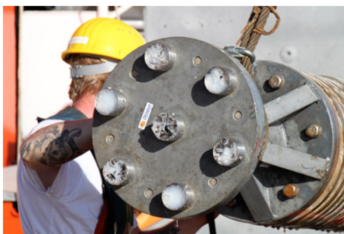
Fig. 4.9.1-2: Rock corer. The shattered pieces of rock stick to the small containers, which are filled with Vaseline and demonstrate a successful sampling of the volcanic crust.
