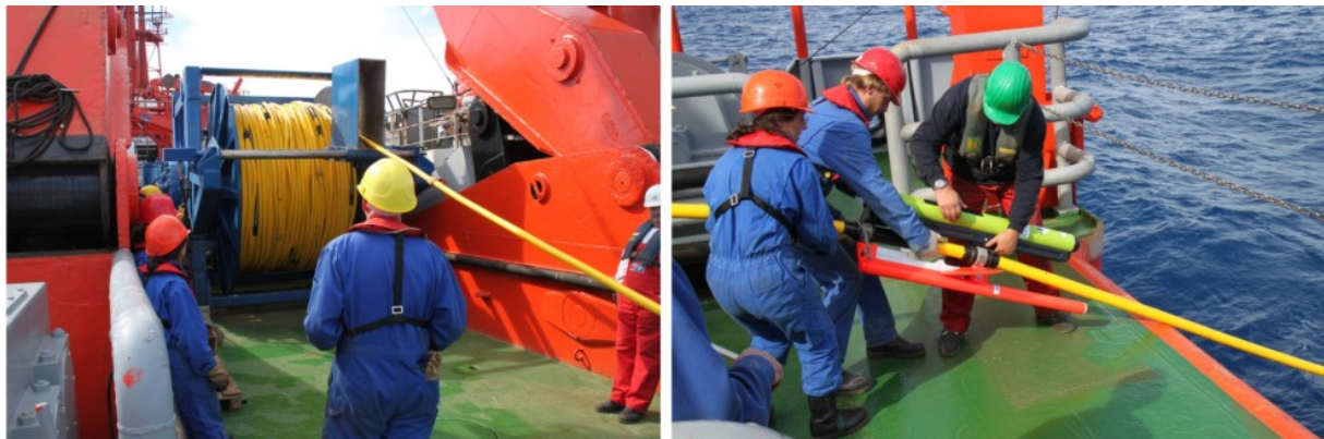
Fig. 4.8.1-2: Deployment of the 3000 m long digital streamer (Type SERCEL), and montage of the Digibirds and rescue system (Photos: T. Ronge).
