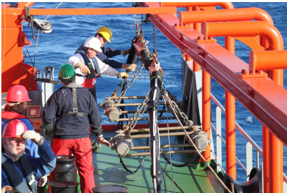
Fig. 4.8.1-1: Two high frequency 2 GI-Airgun cluster used for the seismic surveys (Photo: T. Ronge)
