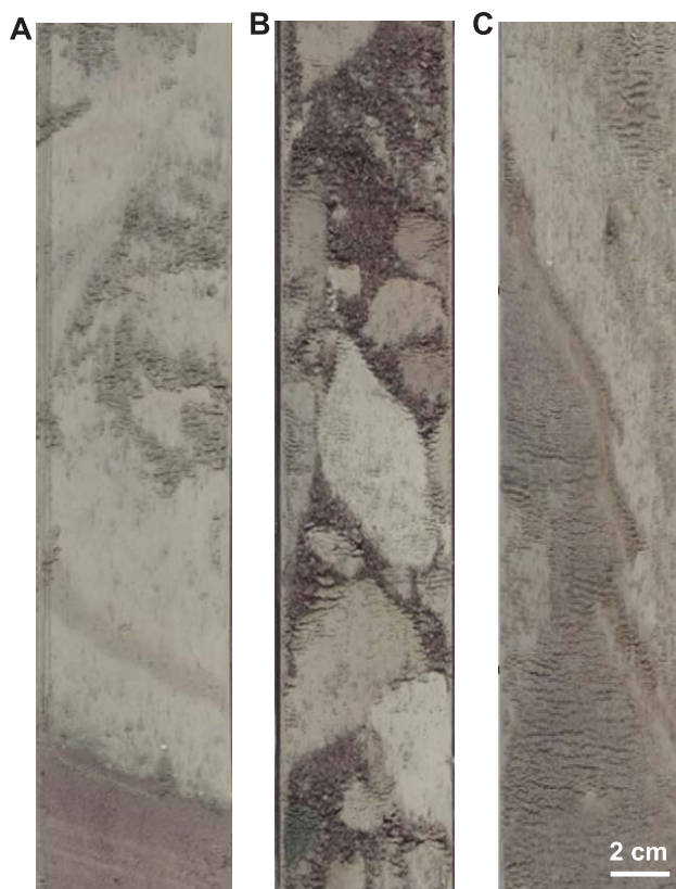
Figure 6. Deformation observed within the cores: (a) Convolutes, U1399A (depth: 25.40m); (b) Mixing, U1400C (depth: 25.05 m); (c) Inclined layers and microfaults; U1400C (depth: 34.95 m).
