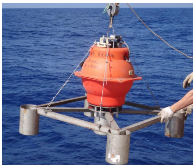
Figure 1. Deploying the I-4C OBS
