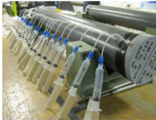
Fig. 14 Pore water sampling from 1 m cores using Rhizon 5 cm samplers connected to 10 ml Luer Lock syringes.
