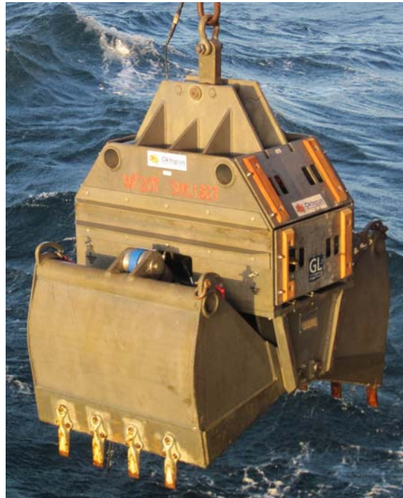
Fig. 15 The GEOMAR video guided hydraulic grab (VGHG) deployed from RV METEOR during cruise M84/5
