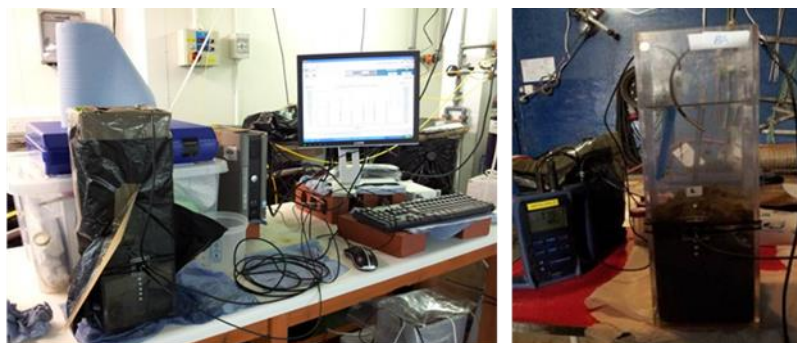
Figure 2: Acquisition of sedimentary pH profiles. Left: aquarium housing sediment and optical sensors (white), connected to a PC. Right: acquisition of optical pH profile using optical sensors at T2, showing temperature sensor (black), and handheld pH macroprobe.
