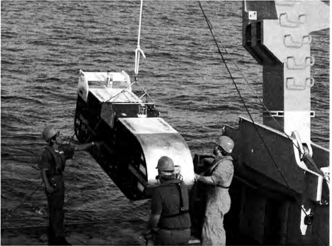
Figure 3.3: The DTS sidescan sonar vehicle during deployment onboard R/V POSEIDON.
