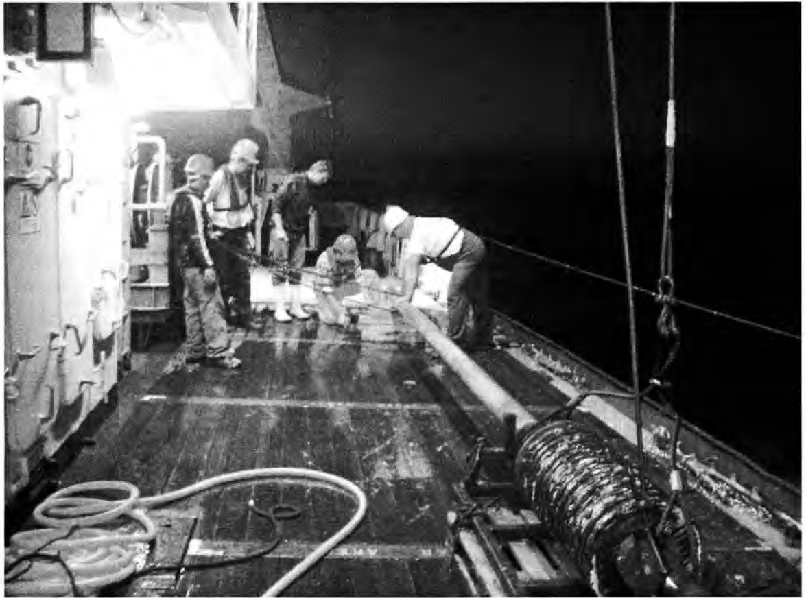
Figure 3.1: The 6-m long gravity corer used during the R/V POSEIDON cruise P317/4.
