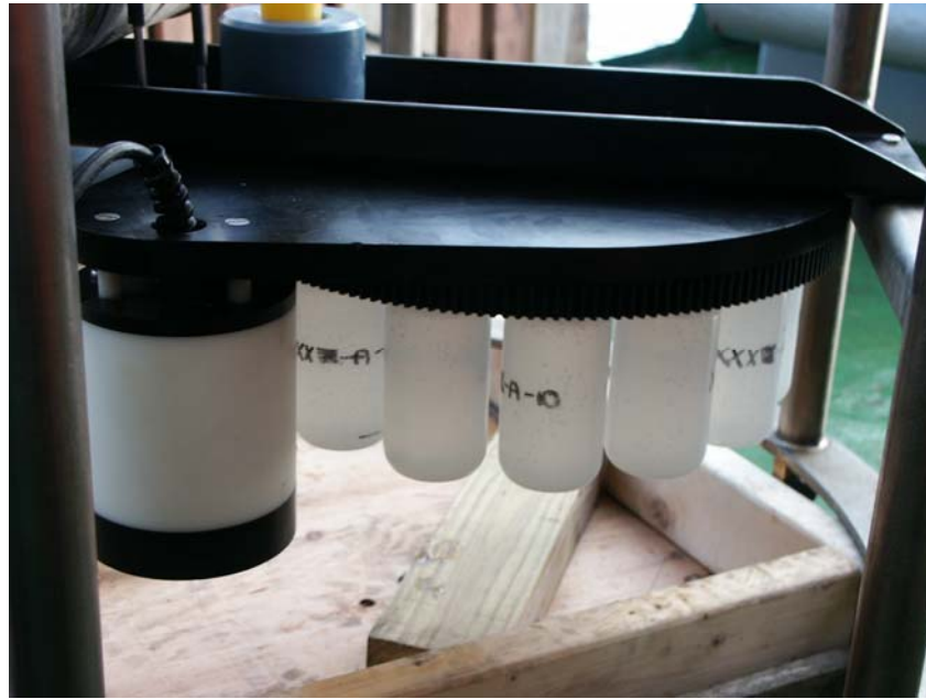
Figure 8: ANIMATE sediment trap from SOC (McLane SN 532).
