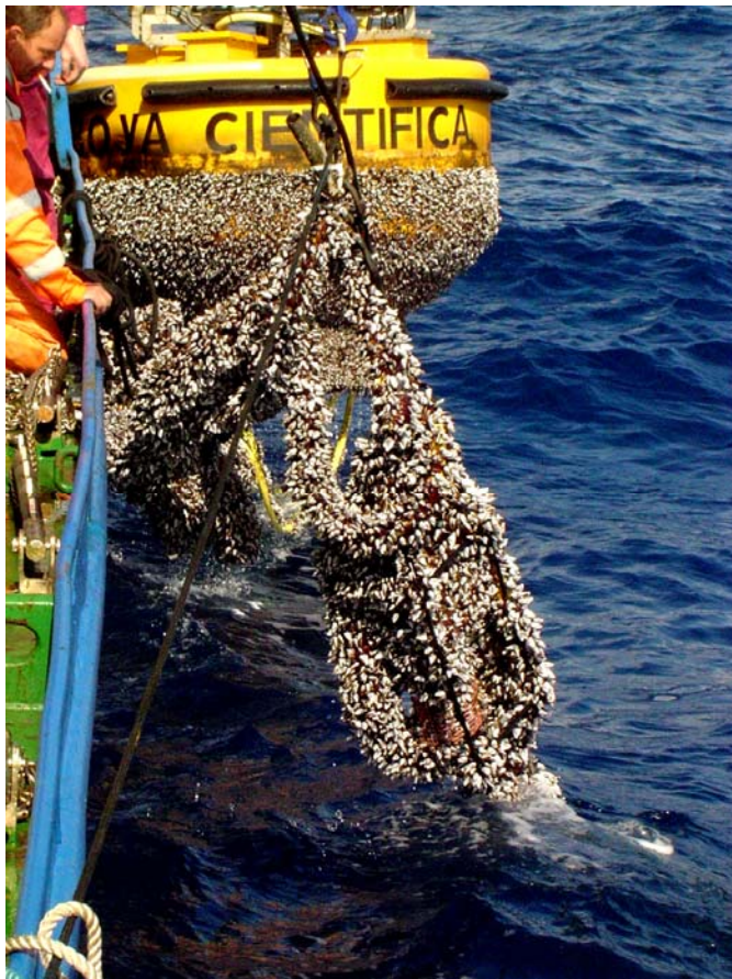
Figure 6: SBU and SAMI sensor with heavy bio fouling.
