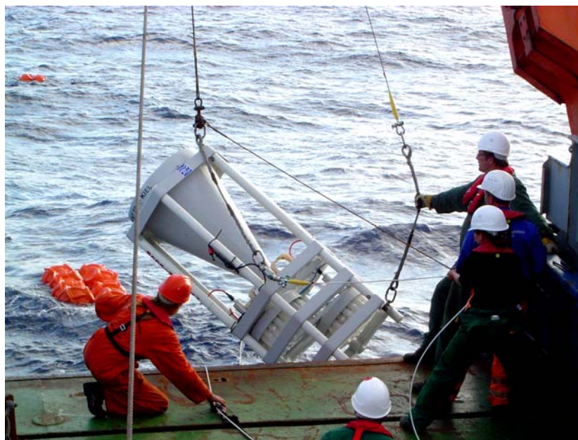
Figure 3: Deployment of the MSD trap, fitted into the ACI-4 mooring array.
