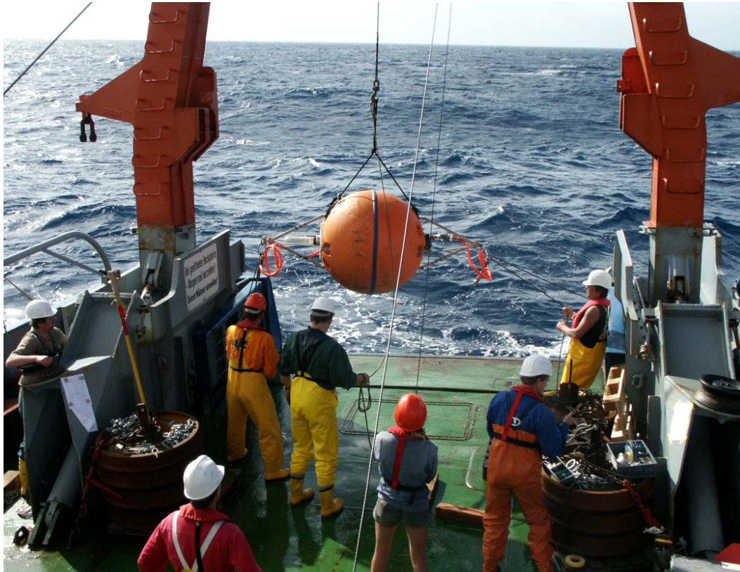
Figure 10: Deployment of the floatation sphere telemetry.
