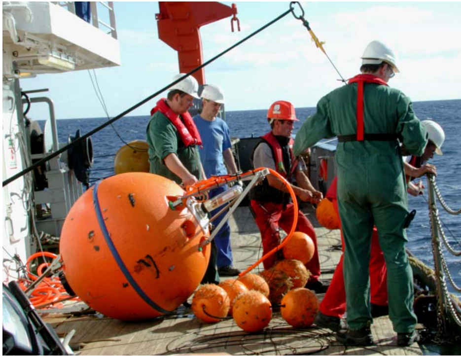
Figure 13: Recovery of the ACI-4 mooring array.
