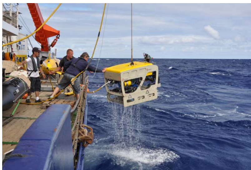
Fig. 8 Recovery of ROV Cherokee after a dive on the western flank of the small Menez Gwen volcano.
