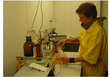
The previously prepared water samples pass through the chemical process of titration to determine the content of oxygen (Metrohm 686 Titroprocessor / Metrohm 665 Dosimat)
