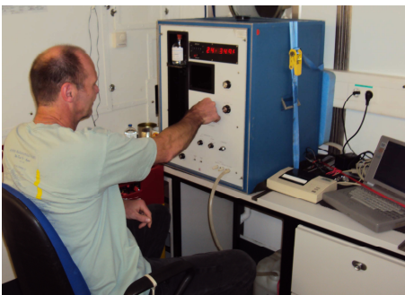
The salinity of the water samples is determined by means of a Salinometer (Guidline Autosal Model 8400A)
