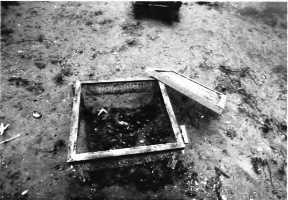
Photo 4. Mussel clump transplantation experiment: Incomplete (roof) cage with vexar mesh as substratum type in 2 m depth after 8 mo of exposure. Stainless steel meshes were regularly cleaned with a wire brush.
