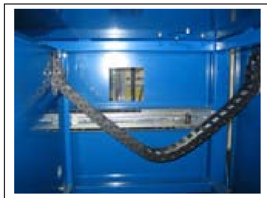
Fig. 5.4 Energy chain connected to the electrical cabinet
