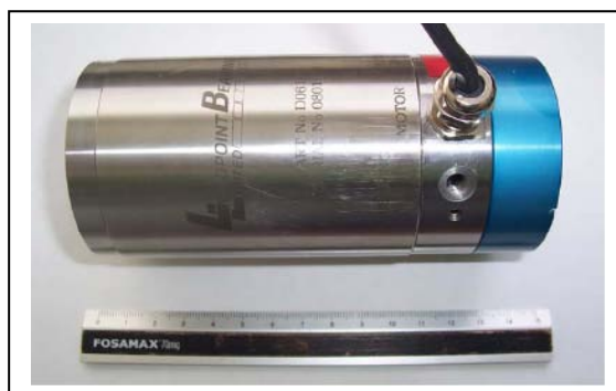
Fig. 3.6 Brushless DC motor driven aerostatic high-speed spindle
