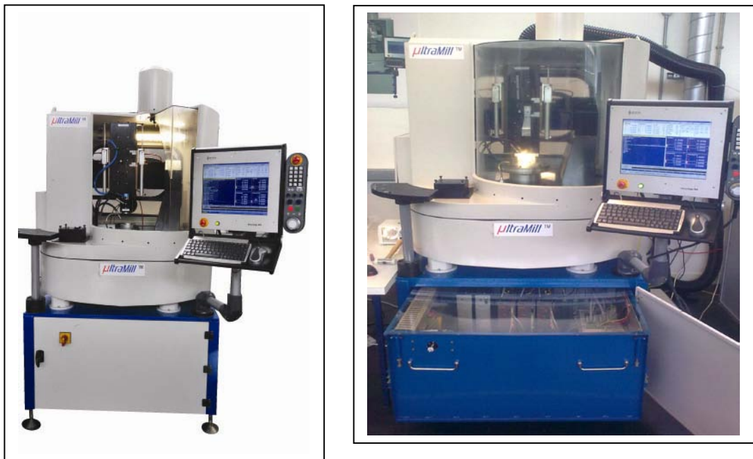
Fig. 2.7 5-axis benchtop micromilling machine (Ultra-Mill, 2009)
