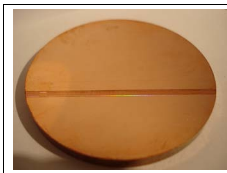
Fig. A-8.9 CVD milled trench with optical surface finish
