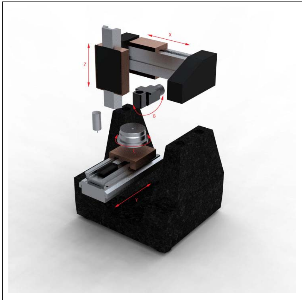
Fig. 3.3 Exploded view of the Ultra-Mill.
