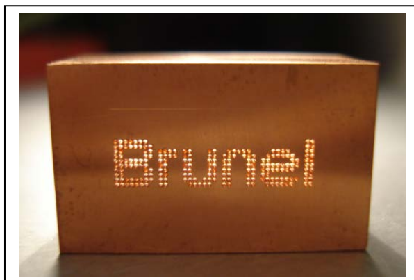
Fig. A-8.8 Micro drilling (200 \mu\text{m} carbide tools)
