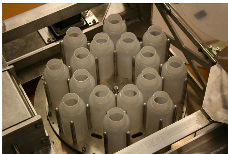
Figure 2: Photograph of sample bottles in the programmable rotating carousel. This carousel can accommodate up to 16 sample bottles, eight of which (interior ones) collect microlayer samples from the glass disk array, while the other eight (exterior ones) collect sublayer water from 0.5 m below the surface. The start time of filling and the filling time are independently programmable for each of the eight bottle pairs.
