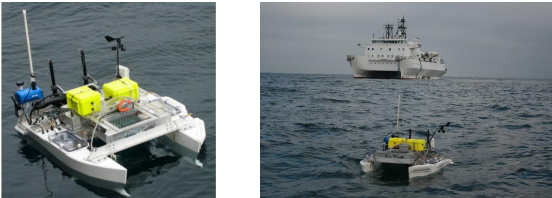
Figure 1: a) Photograph of the radio controlled vessel with rotating disk microlayer sampler and b) R/V Kilo Moana and the microlayer sampler off Santa Barbara, California (courtesy of Masaya Shinki).
