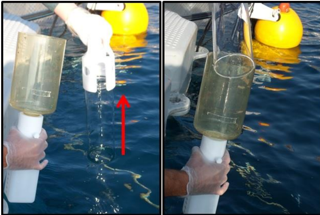
Figure 2: Microlayer sampling with a pure fused silica (quartz) glass tube (Ebling and Landing, 2014).
