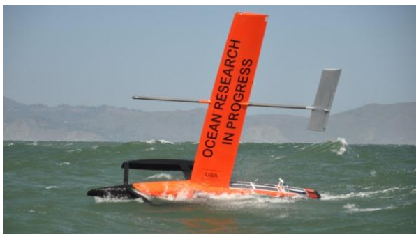
Figure 13: Picture of Sairdrone. Length: 19 ft. Width: 7 ft. Height: 20 ft above water surface. Draft: 6 ft below water surface. Average speed: 3-5 knots. Maximum speed: 14 knots. Payload power available: 5-10 W. Deployment duration: 6-8 Months.
