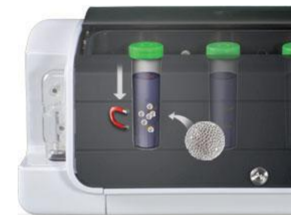
Schematic representation of the incubation chamber with magnetic separator
