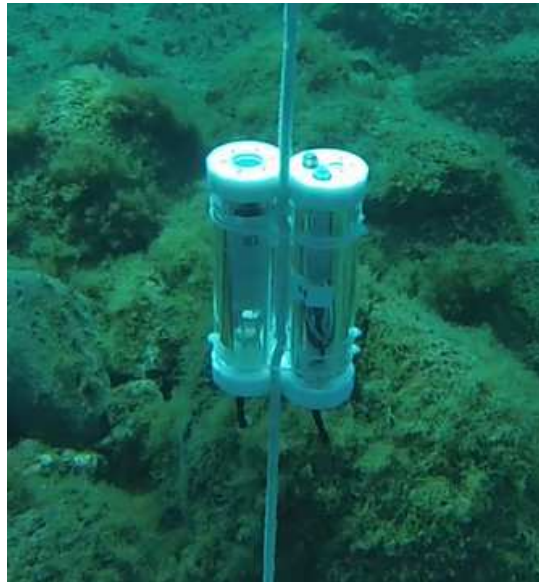
Figure 6. Photograph of the side-by-side deployment of two GasPro sensors, one standard unit for pCO 2 analysis only (left) and a new prototype with a small membrane, a temperature sensor, and a pH sensor mounted together on the front face (right).
