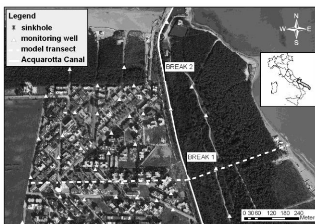
Figure 1: Lesina Marina study area: sinkholes (last updated in March 2012) and monitoring wells locations; white dashed line shows the model transect
