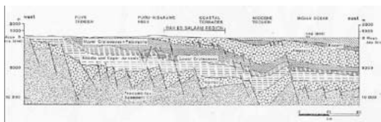
Figure 2 - A geological cross section of the study area (Msindai, 1988)
