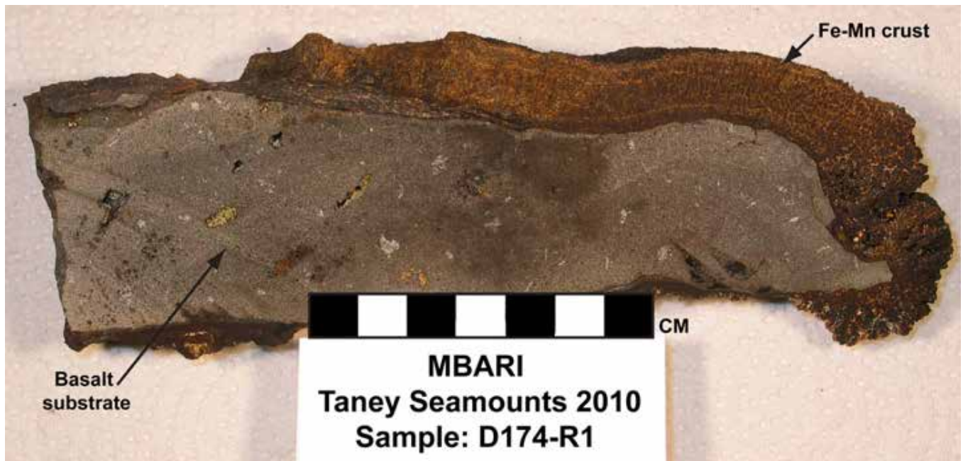
Ferromanganese crust on basalt substrate, collected during Monterey Bay Aquarium Research Institute (MBARI) cruise to the Taney Seamounts – a chain of four undersea volcanoes that lie about 300 kilometres due west of Monterey Bay, California – from August 5–13, 2010 (see http://www.mbari.org/expeditions/Taney10 )
