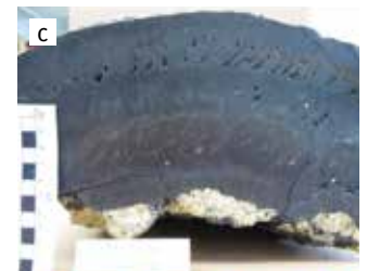
a: The seabed at 2 000 metres water depth showing ferromanganese crust pavement (~4 m by 3 m) on Horizon Guyot, Central Pacific. b: 18-cm-thick crust (D11-1) from 1 780 metres water depth within the Marshall Islands EEZ that started growing onto a substrate rock about 70 million years ago. c: A 12-cm-thick crust (CD29-2; cruise F7-86-HW) from the Johnston Island EEZ (USGS, Hein).
