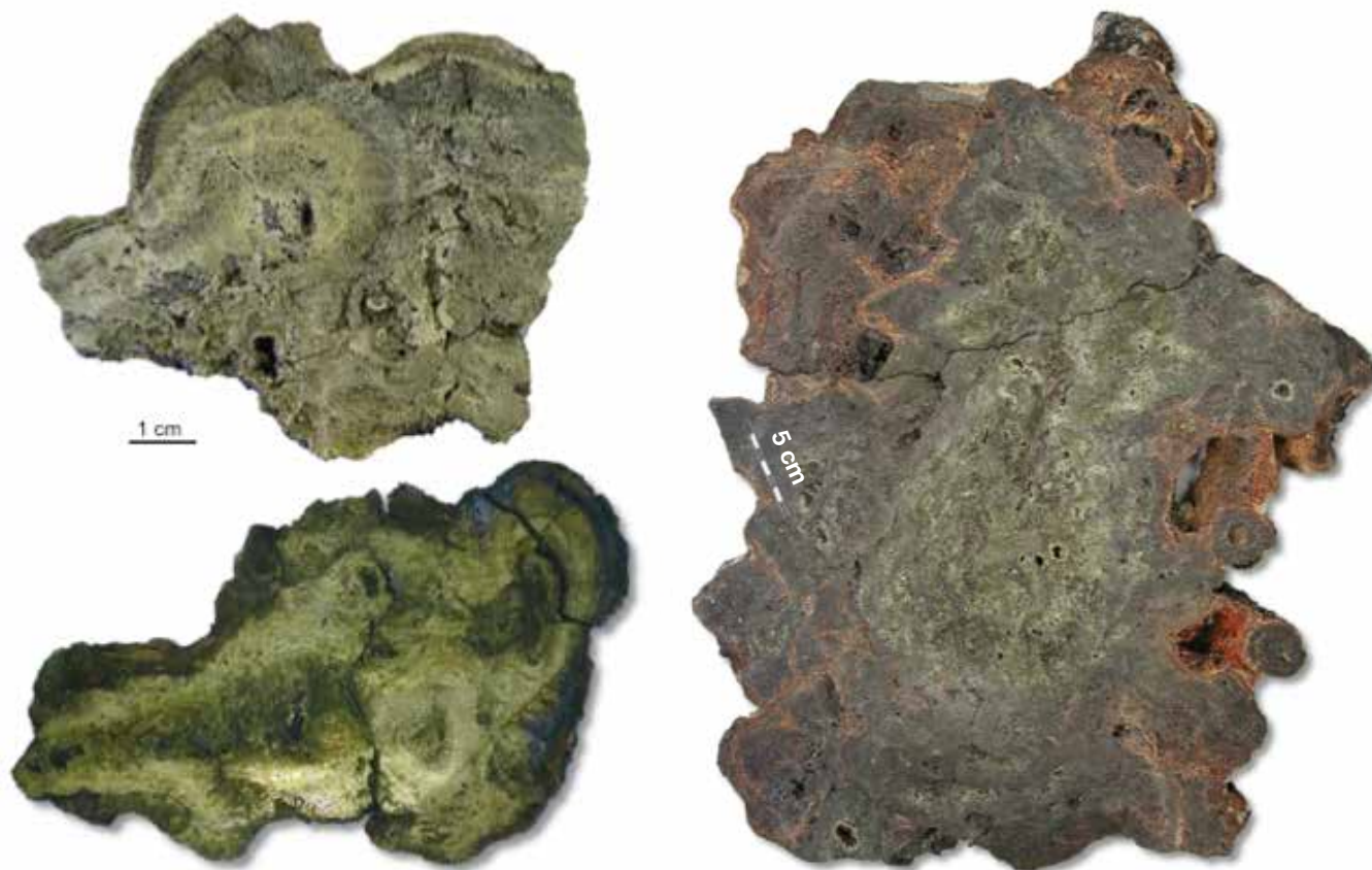
Figure 7. Examples of sea-floor massive sulphides from various tectonic settings. Pyrite-rich chimney from the basalt-hosted Turtle Pits hydrothermal field, 5°S on the Mid-Atlantic Ridge (upper left). A massive chalcopyrite chimney from the ultramafic-hosted Logatchev hydrothermal field (lower left) and a gold-rich copper-zinc massive sulphide from the PACMANUS field, Papua New Guinea. Note the copper-rich core and the brownish zinc-rich exterior of the sample, exemplifying a typical temperature zonation in SMS. Barite constitutes a major part of this sample (right, scale on sample is 5 cm). Photo courtesy of GEOMAR.
