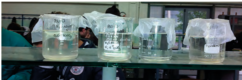
Figure 3. Example of experiment with water added with different nitrate in dark condition. right to left: control (Arno water); 10 ( \text{mg L}^{-1} ) \text{KNO}_3 ; 40 ( \text{mg L}^{-1} ) \text{KNO}_3 ; 20 ( \text{mg L}^{-1} ) \text{KNO}_3 .
