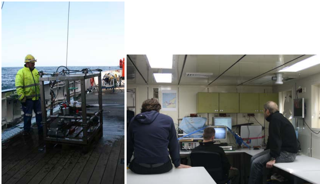
Fig. 5.2.2: (A) OFOS camera system for seafloor observations and gas bubble detection (B) Monitoring the on-line video for gas bubble emission at the seafloor
