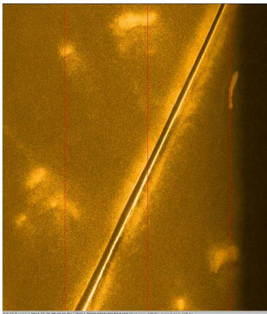
Figure 16: SAS image from the AUV showing shell hash areas and a pipeline. The pictured area is located over the subsurface CO 2 plume.
