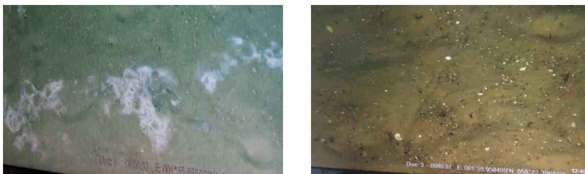
Figure 13: Seafloor images (from ROV) of well 15/9-13 (left panel) and of baseline site 20 m outside well (right panel). Pictures taken from the ROV film.
