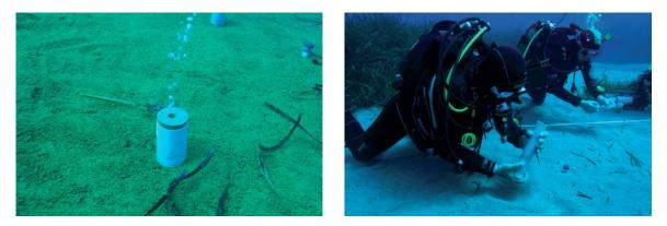
Fig. 5 – Taking sediment samples with push cores and Sarstedt tubes © HYDRA
