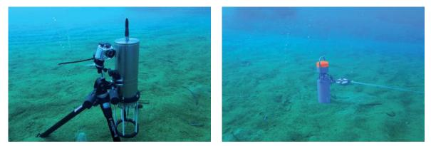
**Fig. 8 – Left: Handheld profiler (right) and camera, Right: SEAGUARD recording current meter** © HYDRA
