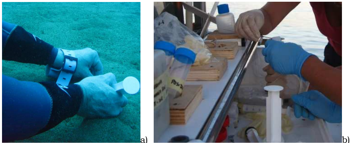
Figure 1. Sampling of sediment by scuba diver (a); extrusion of sediment cores and surface layer subsampling (b)
