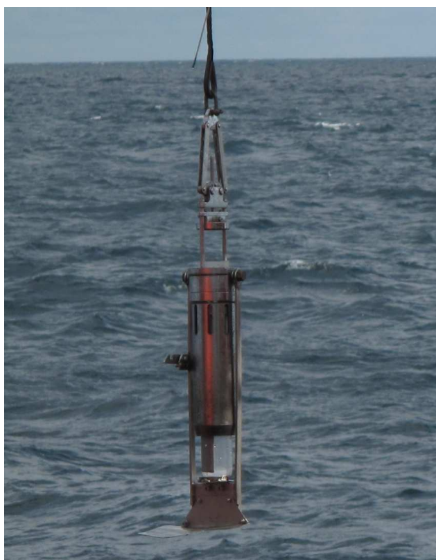
Fig. 12. Niemistö corer used to sample surface sediments and overlying bottom water
