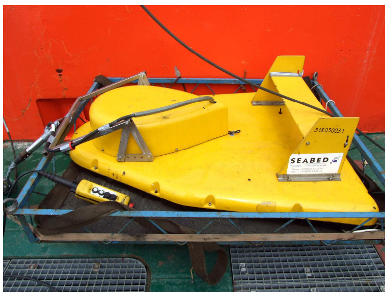
Fig. 3. Chirp subbottom profiler (Edge-tech SB-0512)
