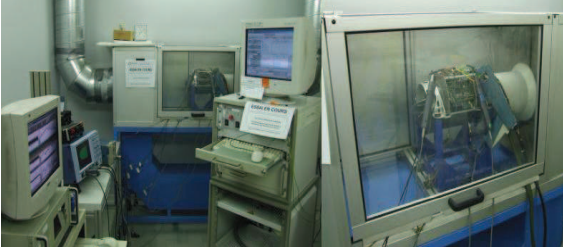
Fig.3. Bearing fault diagnostic setup
