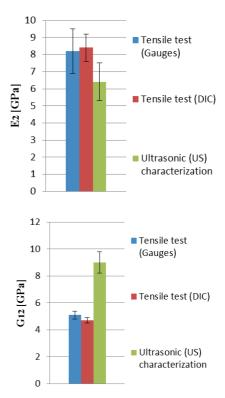
Determination of the elastic properties in CFRP composites: comparison of different approaches...
