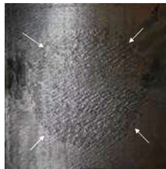
Figure 1. Photograph of the whole axial section of a cubic block 30 cm in size. The white arrows show the limit between the outer non-affected zone and the inner with-CHG area.
