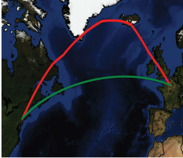
Fig. 2. Difference between the shortest path trajectory (green) and the real trajectory (red) for a Paris-New York flight on the 16 th of September 2011.
