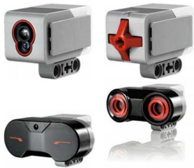
Figure 11: Color, touch, infrared and ultrasonic sensors used for the rendezvous.
