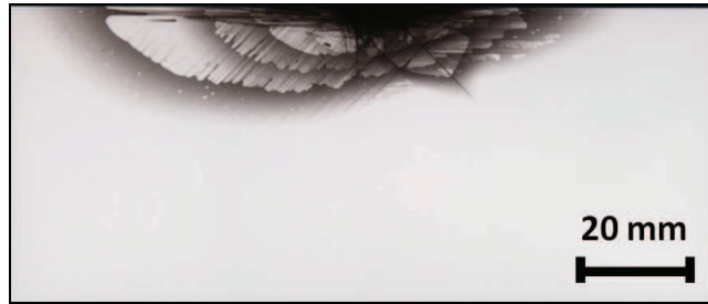
Fig. 9. Stacking 3 XR damage (35 J impact)
