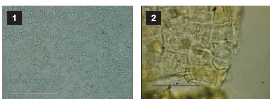
Microscopic sights of hydrophobic phase (1) and insoluble phase (2) (optical microscope Nikon Eclipse E 600, objective with oil immersion, × 1,000).
