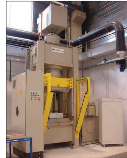
MAPA 400 heated hydraulic press (industrial equipment)
