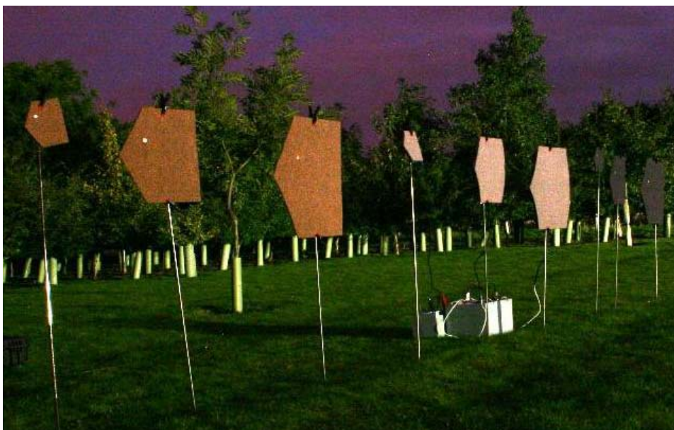
Figure 3.2 Installed targets (light-shaded targets are heated. Lead-acid batteries are below (insulation screen not yet in place))
