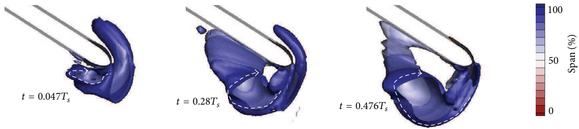
FIGURE 14: Instantaneous isosurface of the negative \lambda_2 vortex criterion representing the vortex formation.
