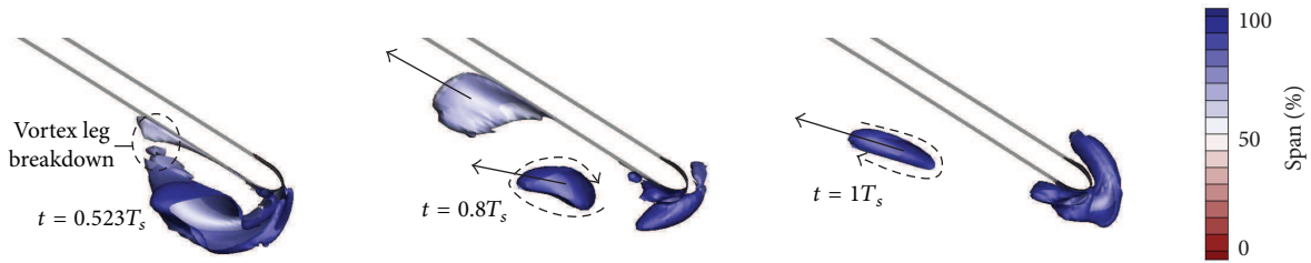
FIGURE 15: Instantaneous isosurface of the negative \lambda_2 vortex criterion representing the vortex displacement.
