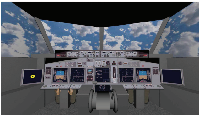
Fig. 4: B737 Layout within CASCaS; Yellow dot marks the current eye-position of the model during simulation (on the leftmost instrument, the EFB)
