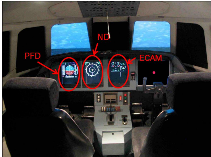
Figure 1 View of the cockpit and the various EFIS. Alerts were displayed in the PFD. The red dot was displayed in peripheral vision on the pilot monitoring PFD screen. ND = Navigation Display; ECAM = Electronic Centralized Aircraft Monitor
