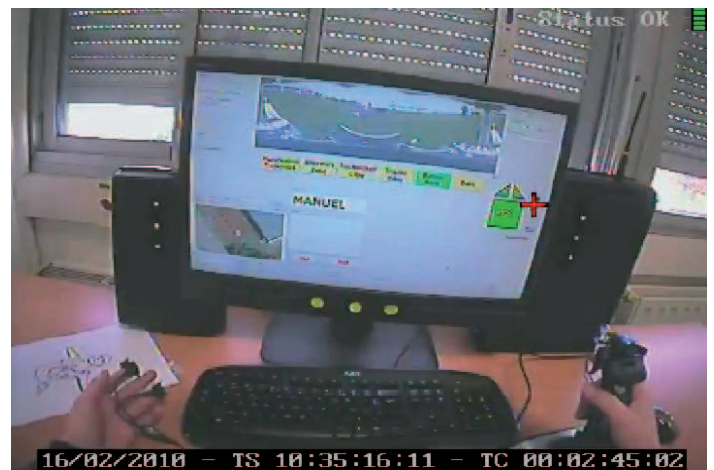
Video 2: the countermeasure disengages the operator's visual focus (red cross) from the panoramic vision and leads him to glance at the battery icon within 1 second. http://www.aerospacelab-journal.org/al4/authority-management-and-conflict-solving
