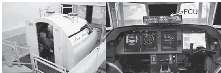
Figure 6. ISAE three-axis flight simulator. Note: Left – outside view of the cabin; right – cockpit view. The arrow indicates the position of the FCU dedicated to program the autopilot (heading, speed, altitude and vertical speed). The participants flew the aircraft from the left seat.
